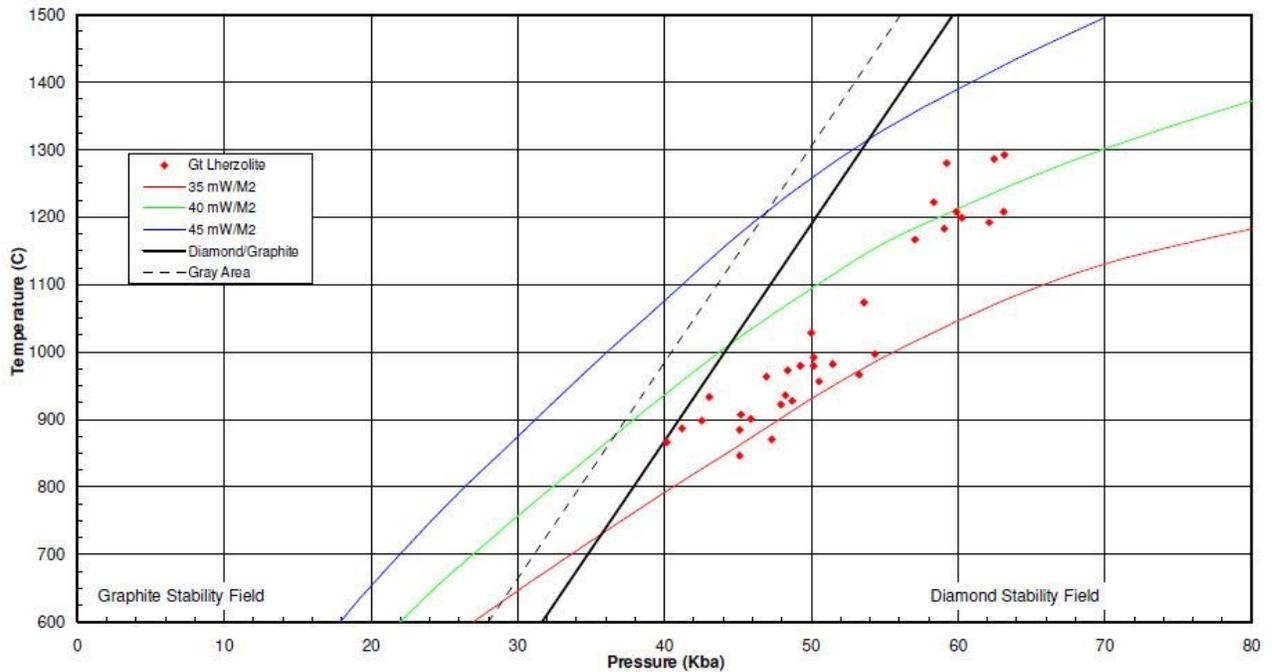
Chrome diopside analyses, when processed using the Nimis and Taylor’s single grain geobarometer shows all CPX analyses plot to the right of the graphite/diamond line. The cluster also plots between 40-45 mW/m<sup>2</sup> as the OPX grains do in the previous section. Below 56 Kba a population with a cooler geotherm is present.
