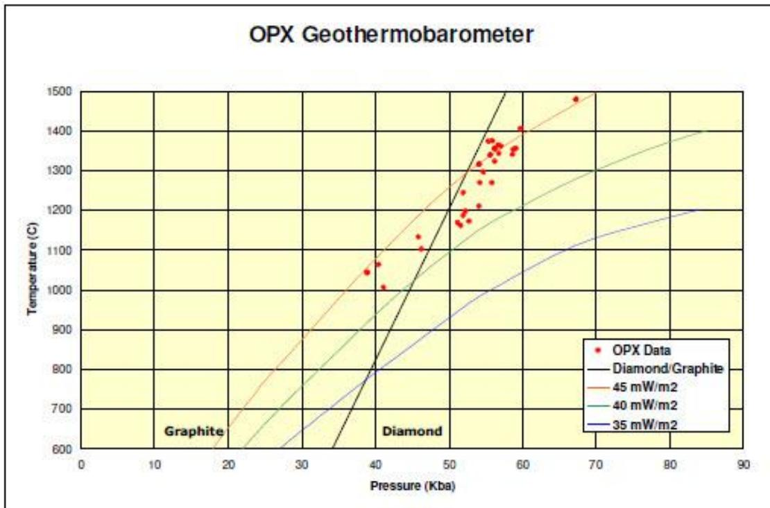
Orthopyroxene analyses align between 40-45 mW/m<sup>2</sup> geotherm with most analyses plotting to the right of the graphite/diamond line. Unfortunately CPX was not present in the database, and I cannot recall if this is a query error, or if CPX was absent (I would guess the first scenario). If DD39 is re-sampled, then CPX should be analysed to see how its geotherm compares to OPX.
