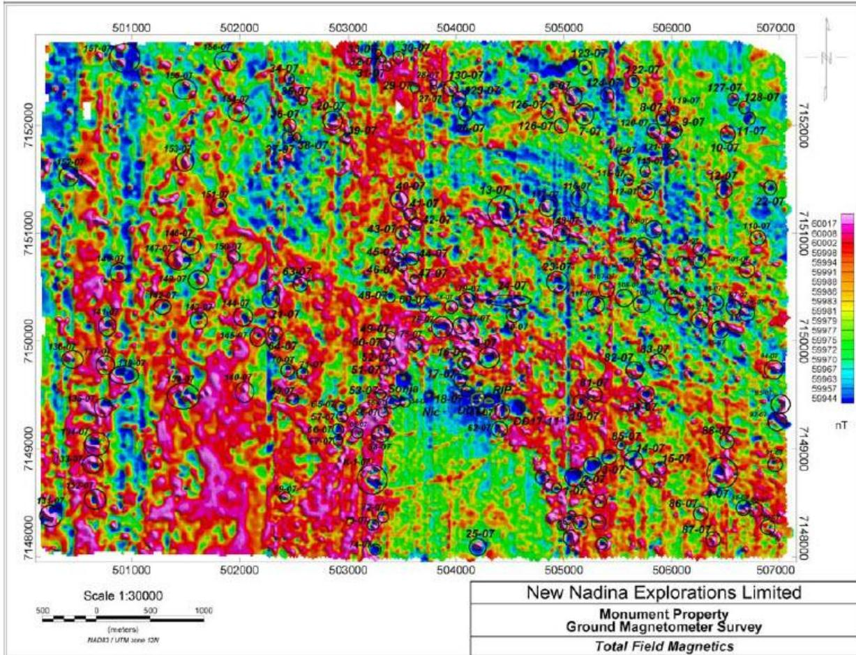
Figure 5. Total Field Magnetics from Sled towed magnetometer survey (Sumara, 2007).
