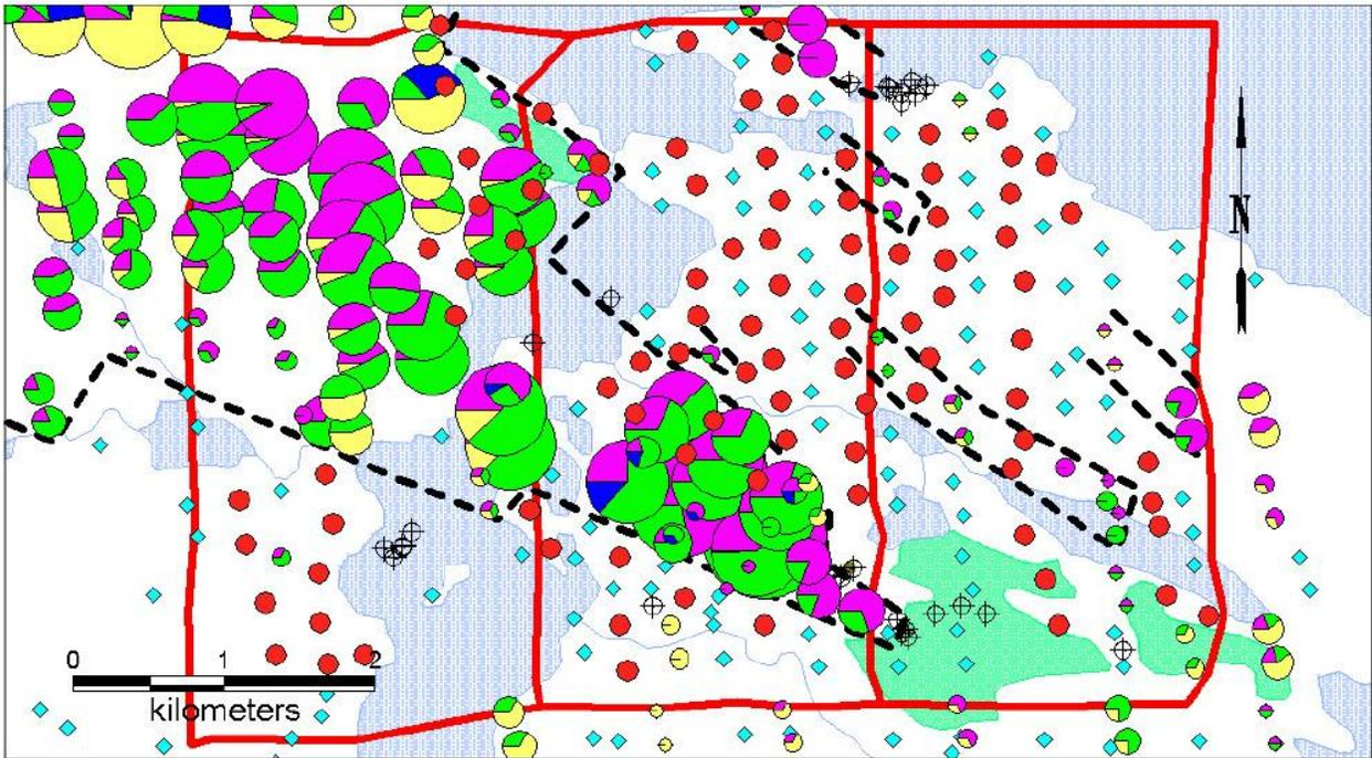
Figure 3. Kimberlite Indicator Mineral (KIM) trains on the Monument Property. Larger circles are higher counts, blue diamonds are zero counts, red dots are proposed samples. Colours code: purple is pyrope, green is chrome diopside, blue is ilmenite and light yellow is olivine. Larger circles represent higher grain counts (from Kivi 2007).
