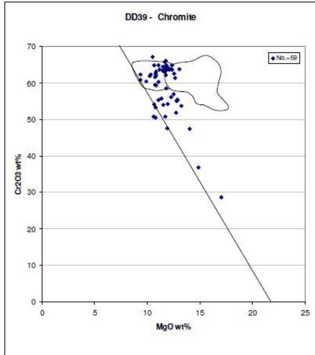
DD39 has a strong representation of high-interest chrome spinel compositions, with at least 7 grains plotting in the diamond inclusion field, and about 18 grains plotting in the diamond intergrowth field to the left. I been a big fan of chromite as a diamond indicator in the central Slave – many kimberlites with only trace diamonds have outstanding chromite chemistry.
