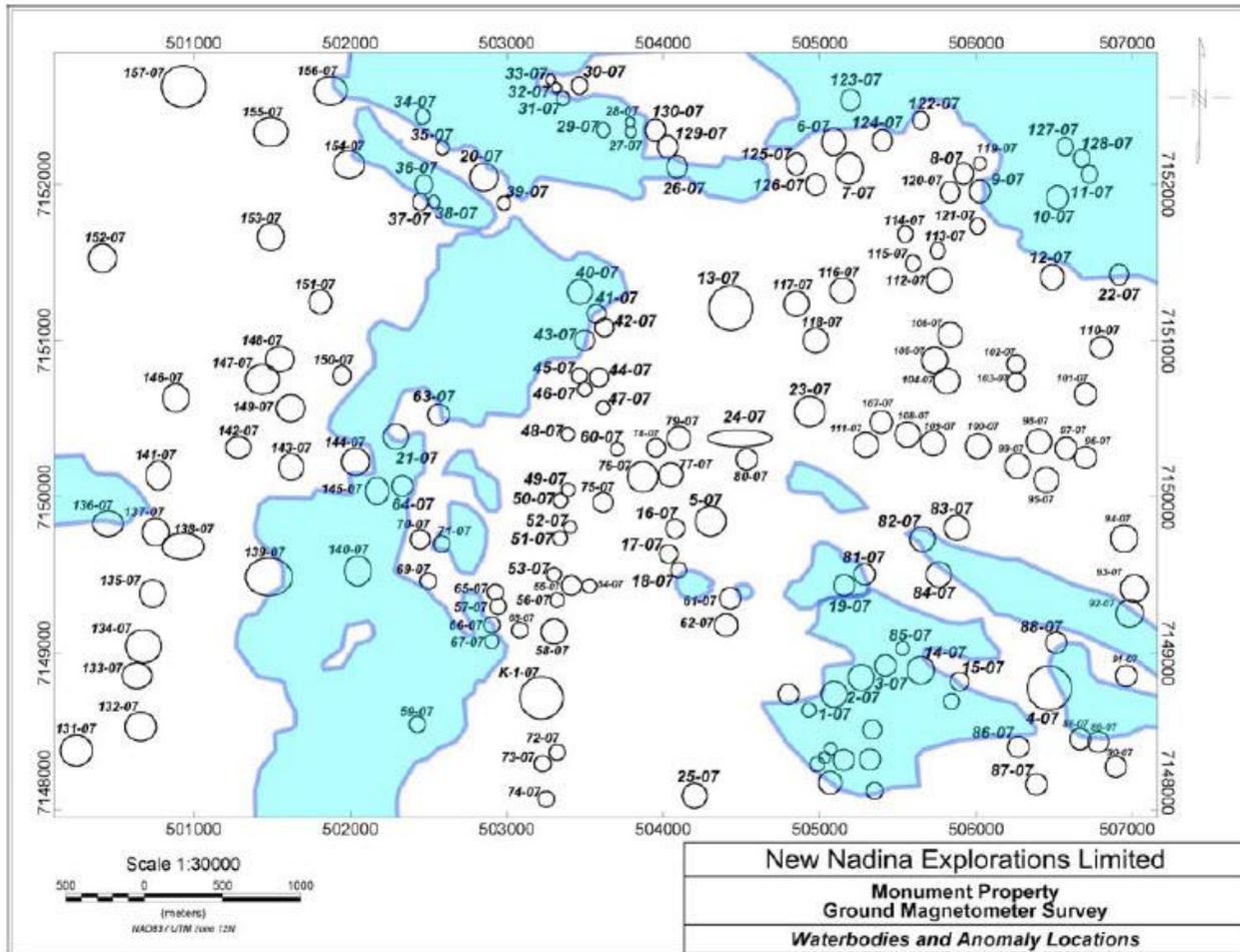
Figure 6. Targets from Sled towed magnetometer survey (Sumara, 2007).
