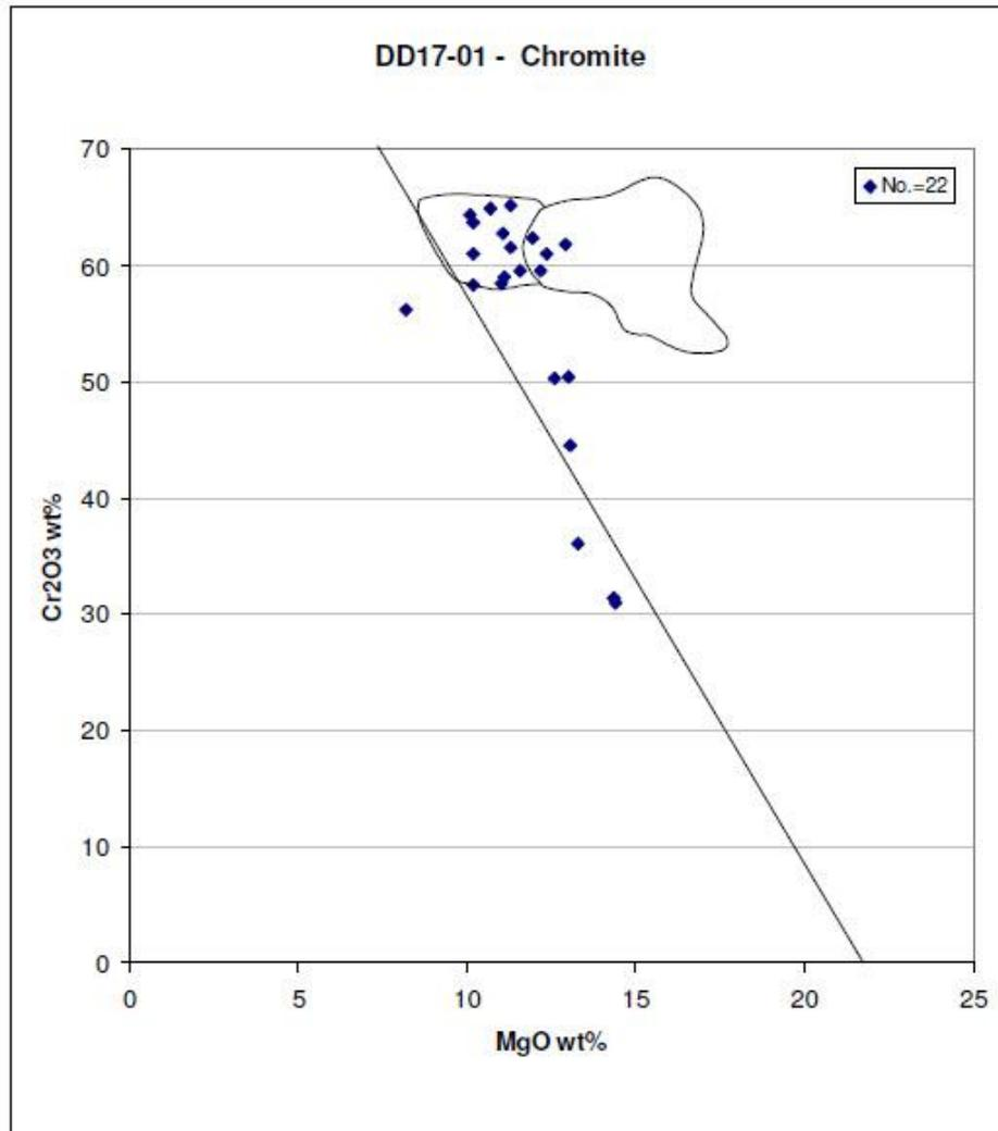
Four chromite grains plot in the diamond inclusion field (right domain) and 12 analyses plot in the domain to the left, which is chromite-diamond intergrowths. The strong representation of high interest
