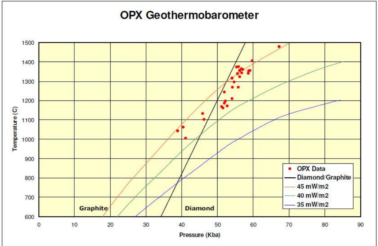
Orthopyroxene analyses align between 40-45 mW/m<sup>2</sup> geotherm. Most analyses plot to the right of the graphite/diamond line. This suggests a significant proportion of the peridotite sampled by kimberlite DD17 is from pressures where carbon would exist in the form of diamond. The small scatter within the graphite field may correspond with low-pressure G-10 pyrope garnets (<6 wt% Cr<sub>2</sub>O<sub>3</sub>).
