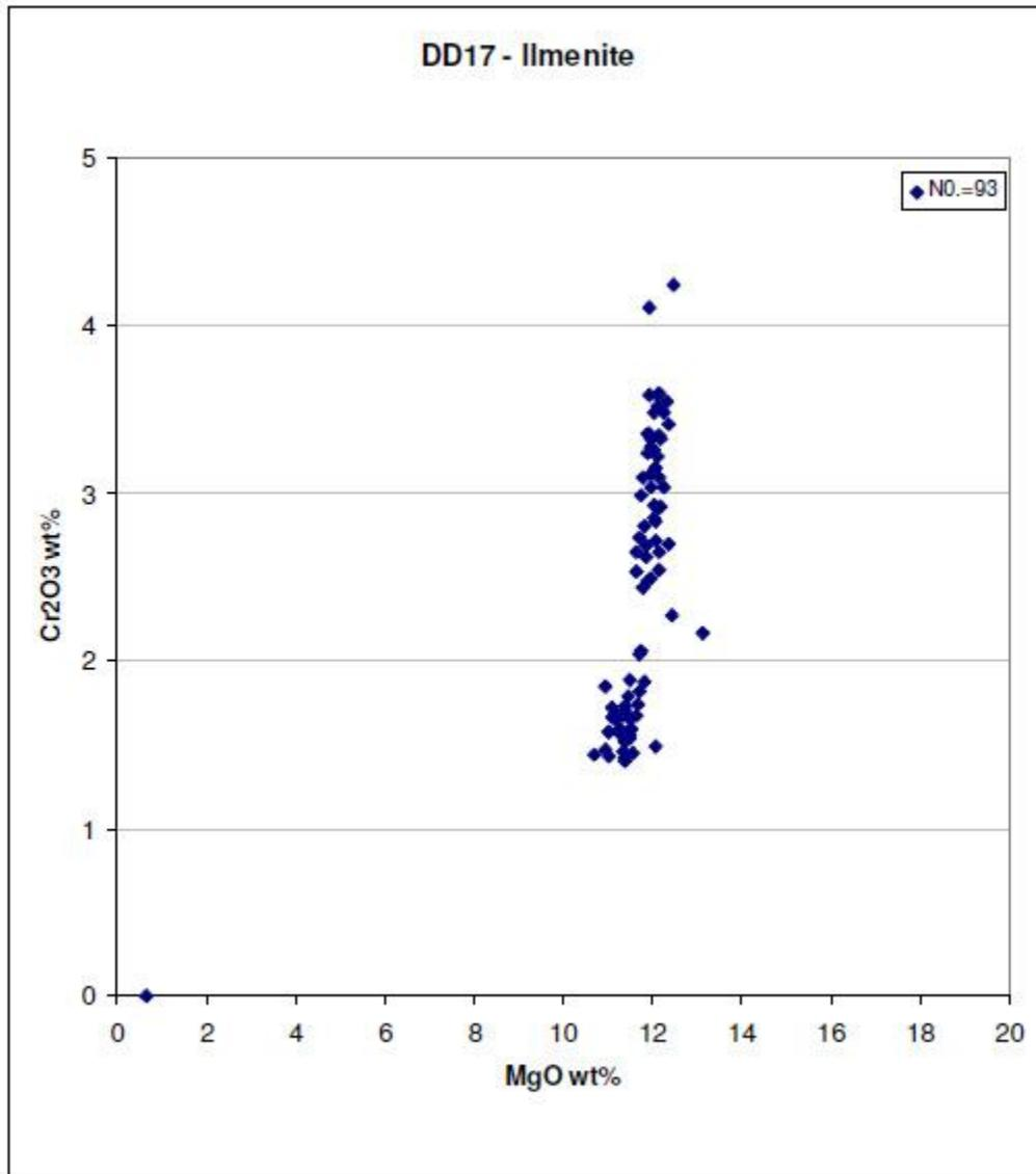
Ilmenite analysed from DD17 show a vertical alignment of analyses which are high in both Cr2O3 and MgO. No Fe-rich compositions are represented. These compositions are favorable for diamond preservation.
