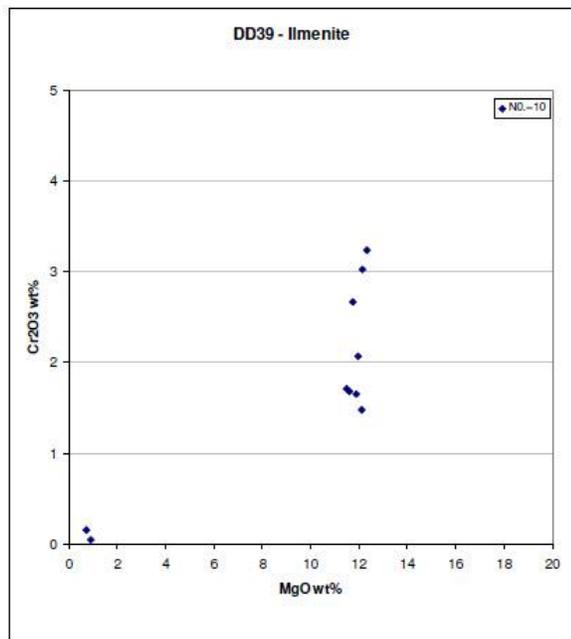
Ilmenite analysed from DD39 show a vertical alignment of analyses which are high in both Cr<sub>2</sub>O<sub>3</sub> and MgO, which is similar to DD17. No Fe-rich compositions are represented. These compositions are favorable for diamond preservation. The paucity of analyses suggest the standard sample was KIM poor.
