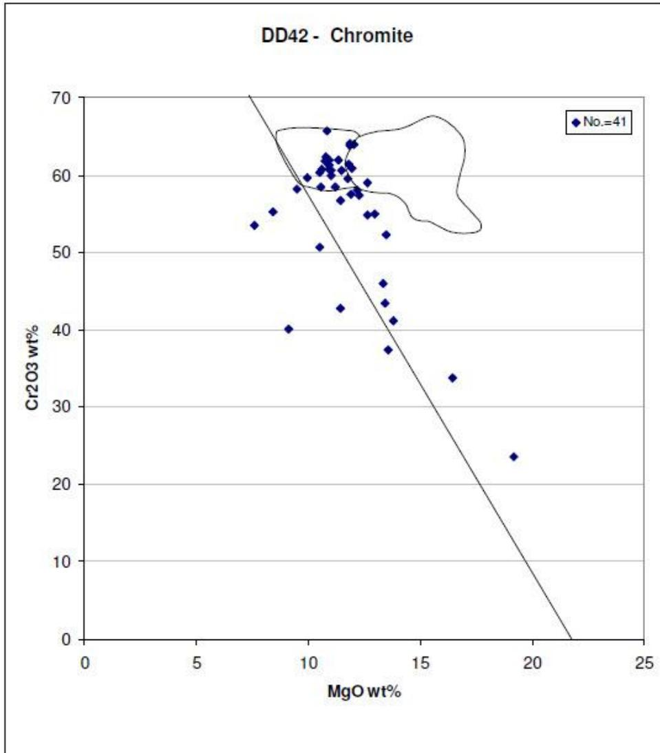
DD42 has a strong representation of high-interest chrome spinel compositions, with 3 grains plotting in the diamond inclusion field, and about 17 analyses plotting in the diamond intergrowth field. I recall that this was the first kimberlite that I saw 50 micron chromite crystals clustered to one another like grapes. I do not know the significance of this texture. Only pyrope and chrome spinel is represented in Kennecott's database.
