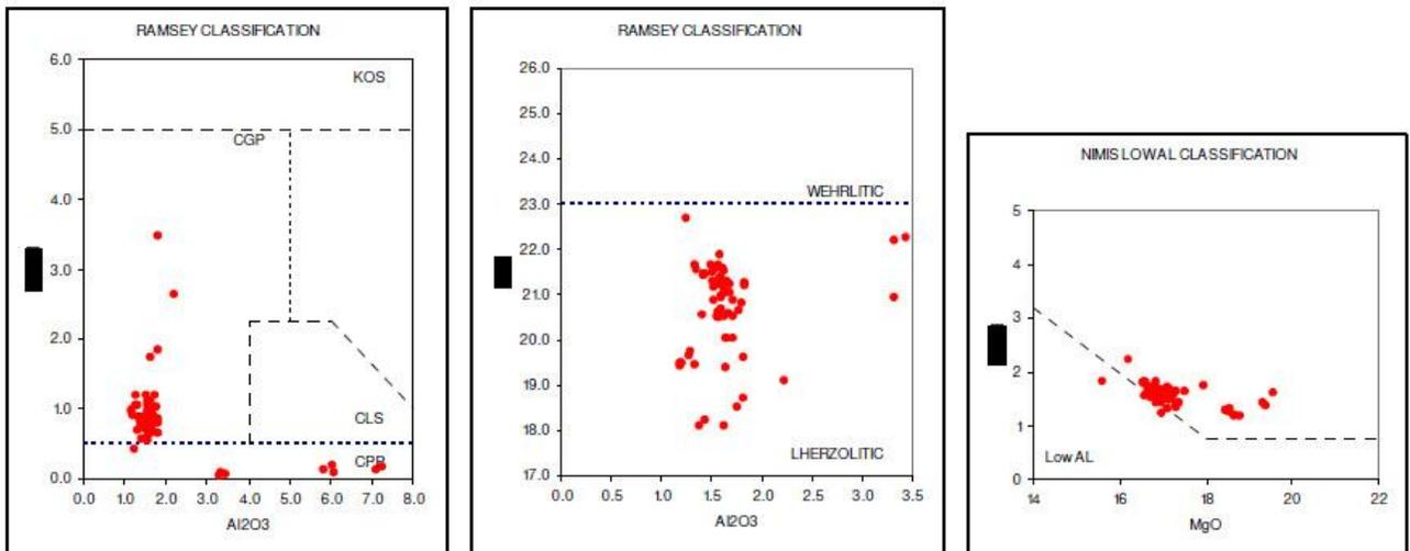
Chrome diopside analyses plotted using Ramsay’s classification shows the dominant source is Iherzolite. Based on the dominant CPX population within the diamond stability field, it is likely that kimberlite DD17 sampled diamond-bearing Iherzolite.
