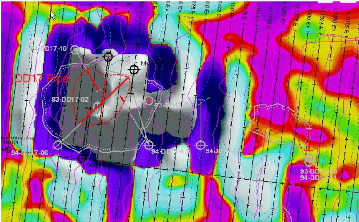
Figure 7. Max-Min 2 HLEM electromagnetic surveys completed by the Monument JV in 2005. Colour gridded data is conductivity; in-phase (solid line) and quadrature (dashed line) profiles are shown along surveyed lines (Kevi 2008).
