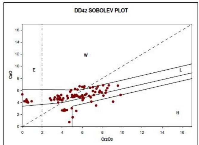
DD42 pyrope garnet shows some similarity to DD17, but the kimberlite lacks high-chrome G9 garnets (> 8 wt% Cr<sub>2</sub>O<sub>3</sub>) and has an abundance of low-pressure G-10s, which suggest that it is sampling too high in the stratigraphy. High temperature eclogite is absent. Two G10 analyses just cross Grutter's diamond line.
