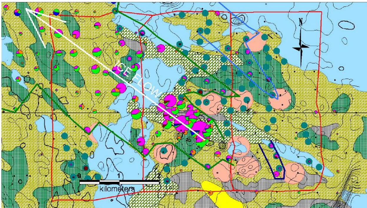
Figure 4. Description after Kivi (2007). Ragged-edged blue pearl KIM dispersal train with several areas of high interest in which a subtle ground magnetic conductor or EM response would be considered a high interest anomaly. Linear counts are represented in pie symbols in Figure 2, whereas a logarithmic count is represented in Figure 1. Teal circles represent 2006 samples, pink circles represent areas of interest.
