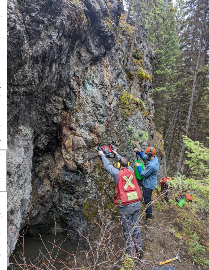
Packsack drilling into Fresh Pots Showing
